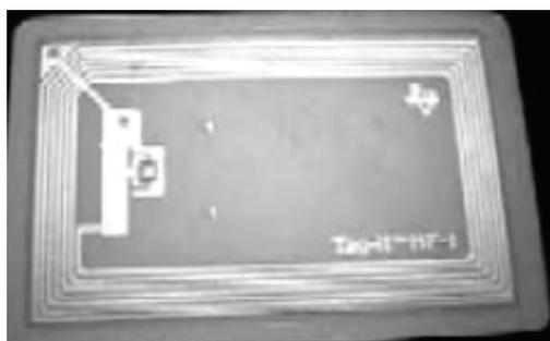
Figura 4. Tag High Frequency (HF) [10].
